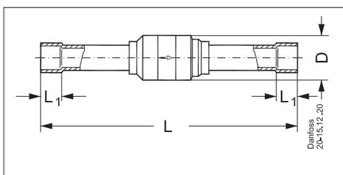
Solder straightway connection - SI Units
